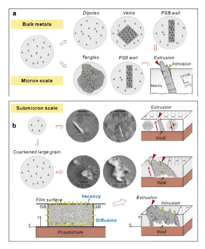
Schematic diagram of fatigue damage mechanisms in metals with different length scales. Credit: IMR
