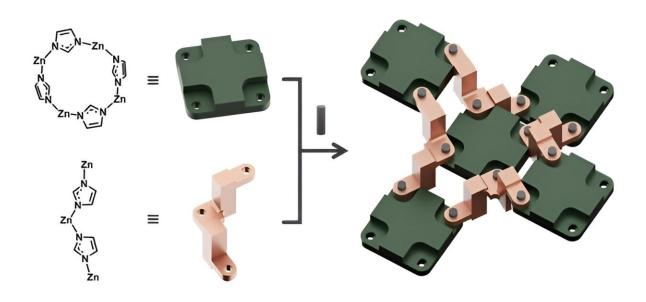
Scheme to build a rotary machine at the molecular scale. Credit: UNIST
