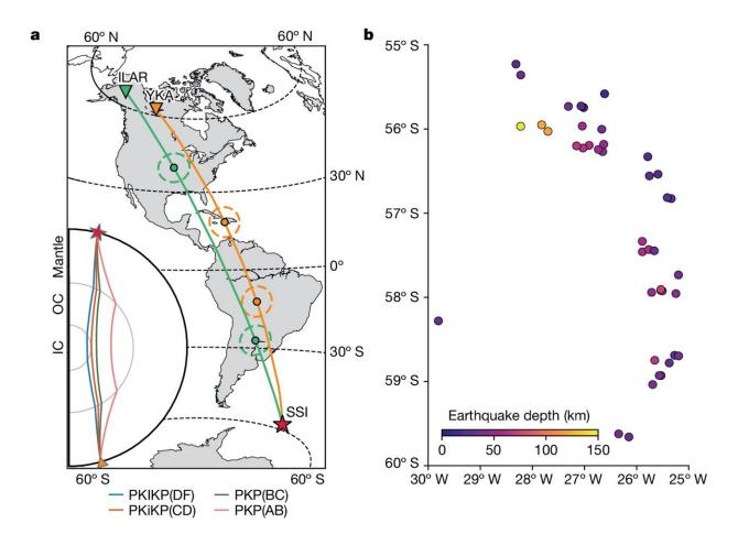
Seismic ray paths and event locations. a, Ray paths of PKIKP and PKP from the SSI source region to the two arrays (ILAR and YKA). The sampled IC region with a representative 1.5 Hz Fresnel zone is marked with dashed circles centered at the PKIKP pierce points at the ICB. Inset, the ray paths of PKP (PKP(AB) and PKP(BC)), PKiKP(CD) and PKIKP(DF). b, Map of the SSI region with the source locations colored by focal depth. Credit: *Nature* (2024). DOI: 10.1038/s41586-024-07536-4
