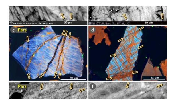
Shocked quartz grains, with fissures filled with meltglass. Credit: UC Santa Barbara
