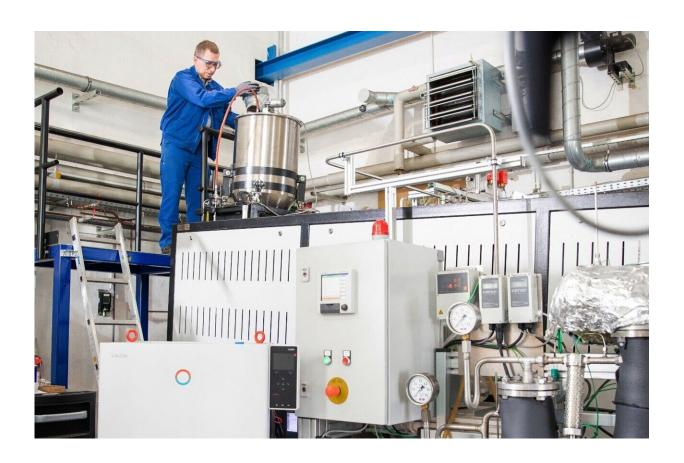
Pyrolysis rotary kilns at the pilot plant scale, with custom-built condensation unit in the foreground. Credit: Fraunhofer IKTS
