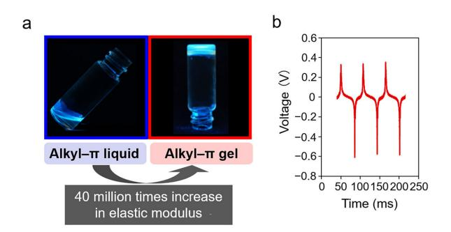
(a) Photographs of an alkyl $-\pi$  liquid and an alkyl $-\pi$  gel in vials. (b) Response of an alkyl $-\pi$  gel-based vibration sensor to 17 Hz vibrations. Credit: Takashi Nakanishi National Institute for Materials Science
