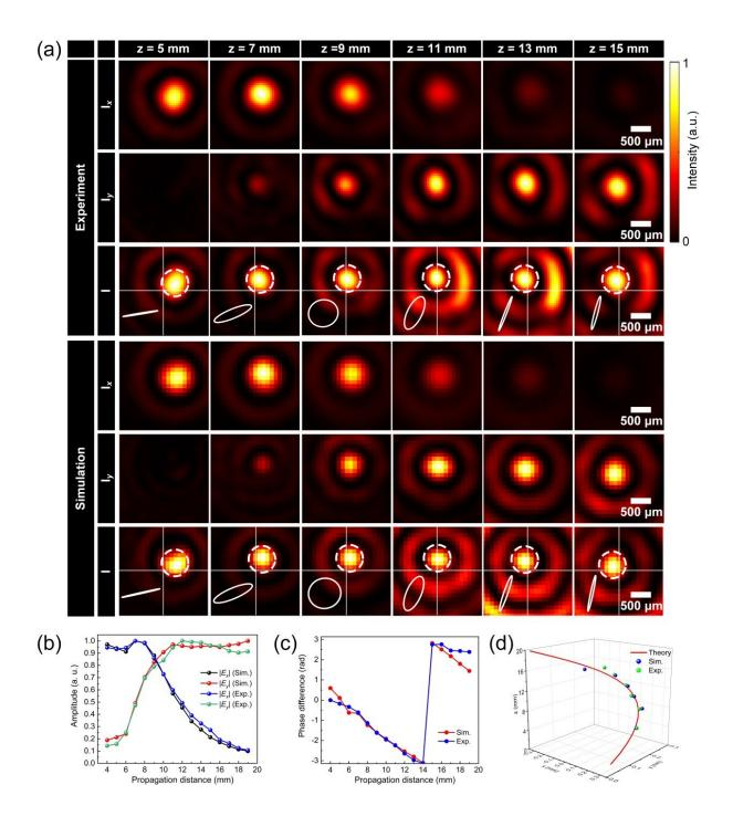
Experimental results of a structured light beam with nonlinear longitudinal polarization variations along a helical transmission trajectory. (a) Intensity distributions for Ex, Ey, and total electric field at different distances. (b) Simulated and experimental amplitudes and (c) phase difference of electric field components Ex and Ey at different propagation distances. (d) Theoretical,
