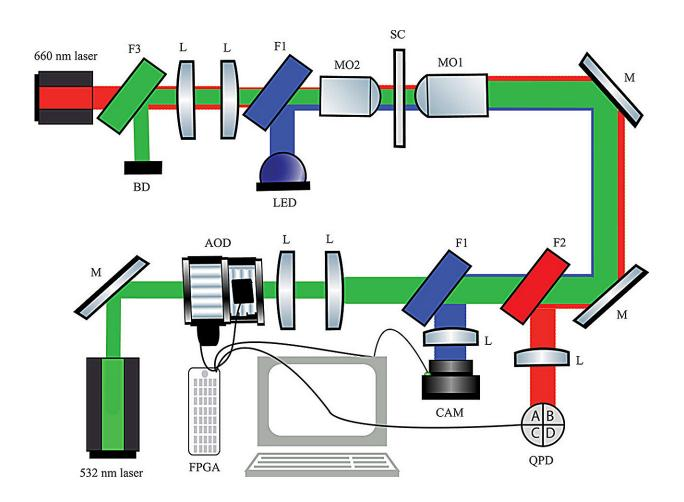
Schematic diagram of the experimental set-up. AOD = Acousto-Optic Deflector, FPGA = field-programmable gate array, QPD = quadrant photodiode, L = lenses, M = mirrors, F1-3 = dichroic mirrors. Representative components are not to scale. Credit: *Advances in Physics: X* (2024). DOI: 10.1080/23746149.2024.2352112
