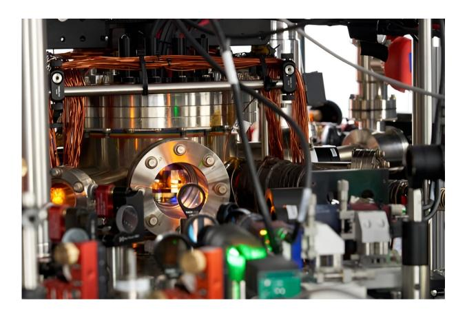
The Will lab uses a series of lasers and optical elements as part of their cooling experiments. Credit: Columbia University
