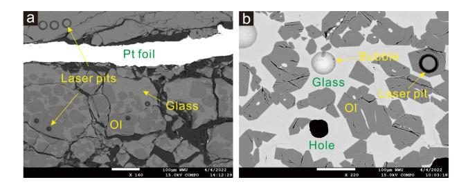
Olivine (Ol) and silicate melt (quenched as glass) were recovered from a gasmixing furnace at 1 atm and 1400 °C. The starting material powders were loaded in a noble capsule and heated in the furnace for 72 hours at different oxygen fugacities. Laser-ICP-MS was used to measure the trace elements in olivine and glass. Credit: Jiejun Jing
