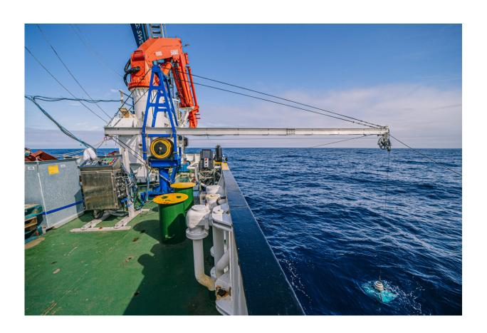
A special high-speed winch that the researchers used to swiftly raise and lower instruments to track the dye's movements underwater. Credit: San Nguyen. Credit: San Nguyen
