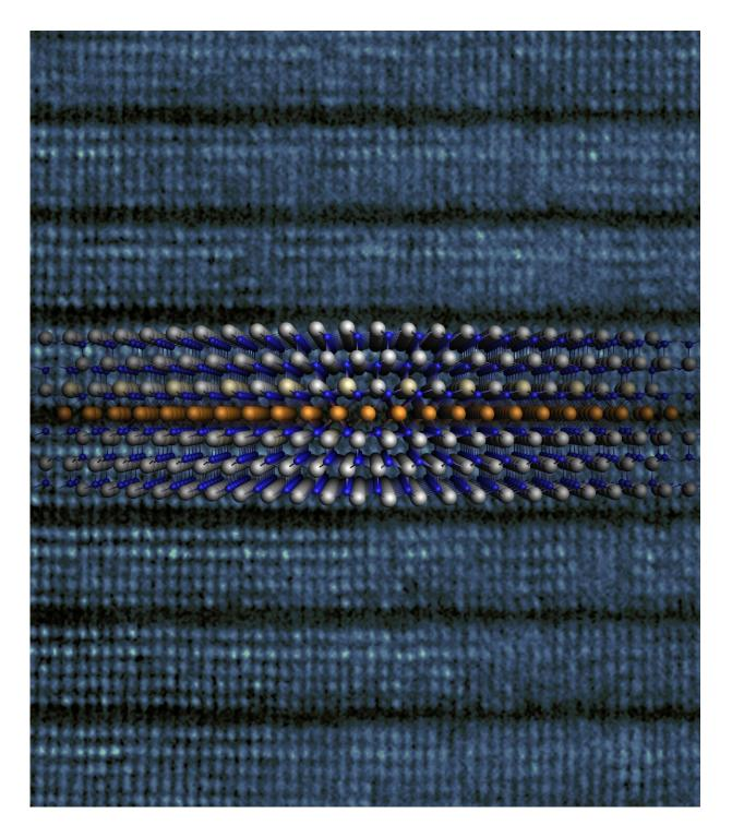
Thermal treating of metallic magneiusm on gallium nitride semiconductor results in the formation of a distinctive superlattice structure. Magnesium, nitrogen, gallium atoms are shown in orange, blue, and gray, respectively. Credit: Jia Wang
