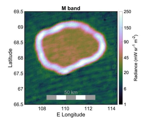
Infrared data collected Oct. 15, 2023, by the JIRAM instrument aboard NASA's Juno shows Chors Patera, a lava lake on Jupiter's moon Io. The team believes the lake is largely covered by a thick, molten crust, with a hot ring around the edges where lava from Io's interior is directly exposed to space. Credit: NASA/JPL-Caltech/SwRI/ASI/INAF/JIRAM/MSSS
