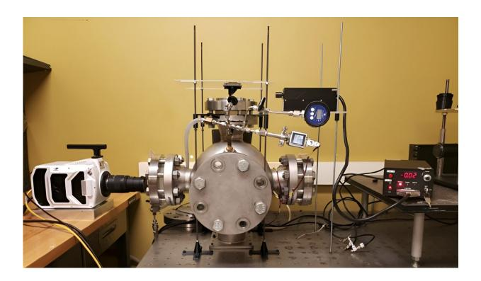
Combustion chamber designed to simulate the lunar environment. Credit: University of Waterloo
