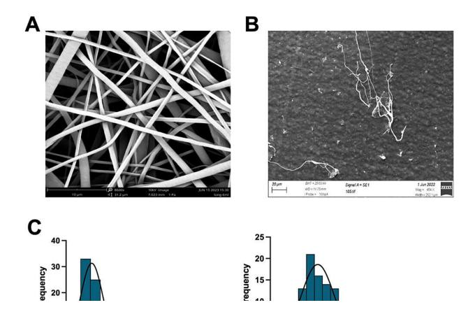
Characterization of nanofibers. (A) SEM images for PCL nanofiber mesh. (B) SEM images for nanoscaffolds. (C) Distribution of the length and diameter of the nanoscaffolds (Taken from 100 different nanofibers). (D) ATR-FTIR for Raw PCL, PCL nanofibre mesh and nanoscaffolds. Credit: *ACS Applied Materials & Interfaces* (2024). DOI: 10.1021/acsami.3c17384
