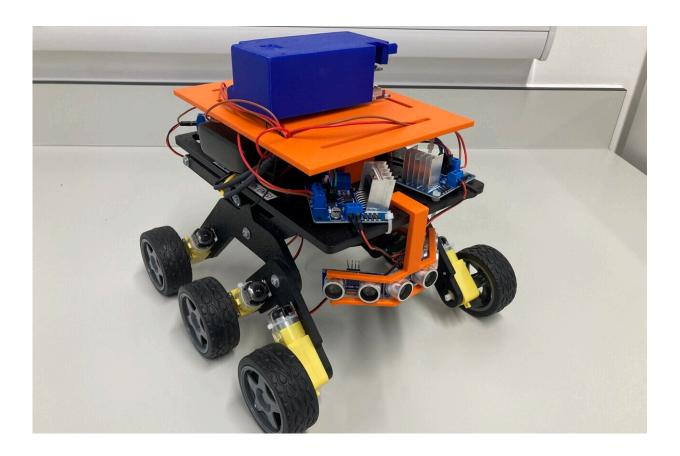
The rocker bogie runt rover has been selected as it has a small form factor and utilises off the shelf components. Credit: Sarah Swinton.
