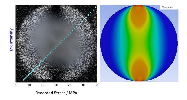
This study represents the stress recording (MR) function of multi-piezo mechanoluminescent material Li<sub>0.12</sub>Na<sub>0.88</sub>NbO<sub>3</sub> through afterglow for the first time. Unlike traditional ML materials that solely enable real-time measurement of mechanical information, the novel MR capability is expected to be highly valuable for capturing the historical distribution of stress. Credit: Tomoki Uchiyama, Chao-Nan Xu et al.
