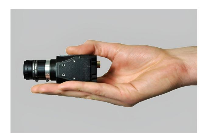
Researchers used inkjet printing to create a multispectral version of a light field camera, which fits in the palm of the hand. The 3D camera could be useful for applications such as autonomous driving, classification of recycled materials and remote sensing. Credit: Maximilian Schambach, Karlsruhe Institute of Technology
