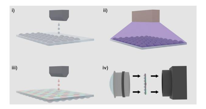
Inkjet printing was used to deposit single droplets of material to form individual lenses on one side of ultrathin microscope slides (i). After curing (ii), fully aligned color filter arrays were printed on the opposite side of the microscope slides (iii). The resulting optical component was integrated directly onto a CMOS camera chip and placed in a camera housing (iv). Credit: Qiaoshuang Zhang, Karlsruhe Institute of Technology
