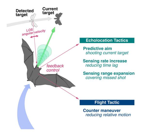
The combination of three echolocation tactics and one flight tactic works to dramatically improve the tracking accuracy. All tactics can be explained as reactive control to the Line of Sight [LOS] angular velocity. Credit: Nozomi Nishiumi
