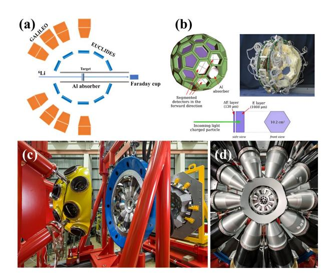
Using the advanced GALILEO Array coupled with the  $4\pi$  Si-ball EUCLIDES, the researchers conducted in-depth spectroscopic analysis to track and identify the reactions. The gamma-gamma coincidence method was crucial in isolating specific reaction channels, allowing the team to pinpoint the behavior of nuclei
