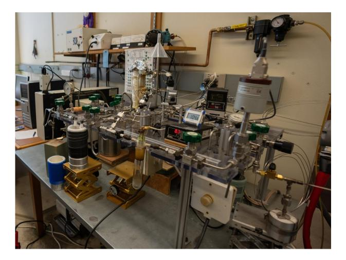
The equipment used to identify the "fingerprint" of magma sources. Called a laser fluorination line, the apparatus extracts and measures oxygen isotopes. This is housed in volcanologist Ilya Bindeman's lab at the University of Oregon. Credit: Charlie Litchfield/University of Oregon.
