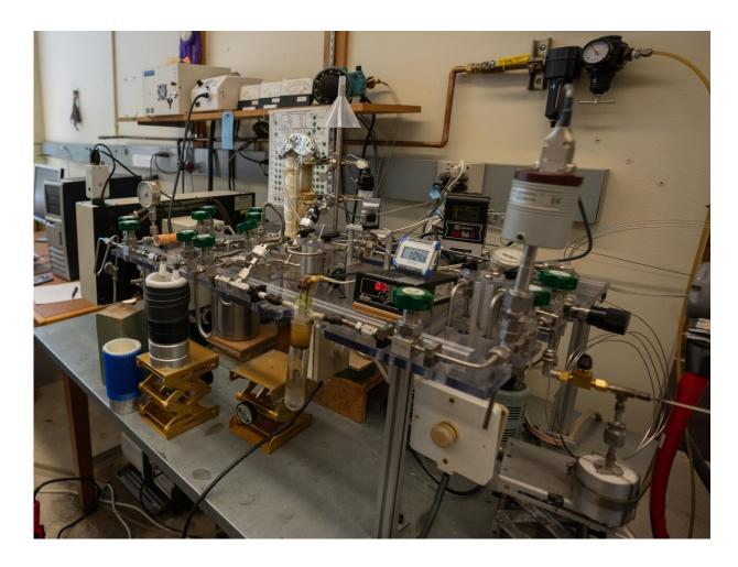
The equipment used to identify the "fingerprint" of magma sources. Called a laser fluorination line, the apparatus extracts and measures oxygen isotopes. This is housed in volcanologist Ilya Bindeman's lab at the University of Oregon. Credit: Charlie Litchfield/University of Oregon.
