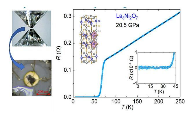
The left image shows the diamond anvil cell used for high-pressure measurements in this study, with the sample surrounded by a pressure-transmitting liquid; the right image shows the resistance curve at 20.5 GPa, a perfect superconducting transition near 66K with zero-resistance below 40 K are presented. Crystal structure of  $La_3Ni_2O_7$  is plotted in the inset. Credit: Zhang et al.
