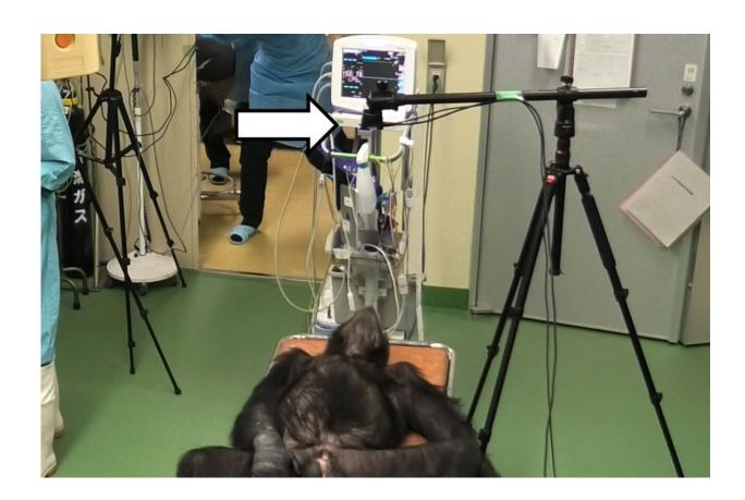
High-frequency radar can detect extremely subtle body movements, such as those caused by the heart beating. In this study, researchers used millimeter-wave radar to remotely measure heart rate in two adult chimpanzees. The results accurately matched those obtained using standard electrocardiography, showcasing the potential of this method. Credit: Takuya Matsumoto / Shinshu University
