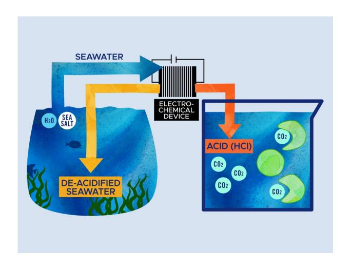
PNNL researchers grew Picochlorum celeri, a fast-growing species of microalgae, in beakers with and without an acid byproduct from the electrochemical removal of acid from seawater. With the acid, the microalgae grew three times faster. Credit: Sara Levine | Pacific Northwest National Laboratory
