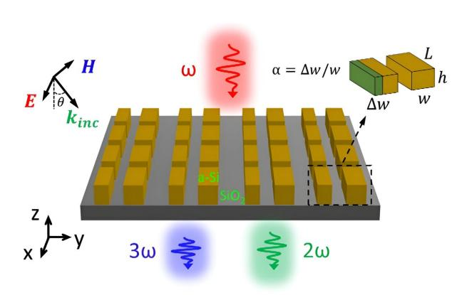
Schematic diagram of a nonlinear metasurface composed of asymmetric metaatoms based on guided mode resonance and bound states in the continuum. Credit: *Opto-Electronic Advances* (2024). DOI: 10.29026/oea.2024.230186
