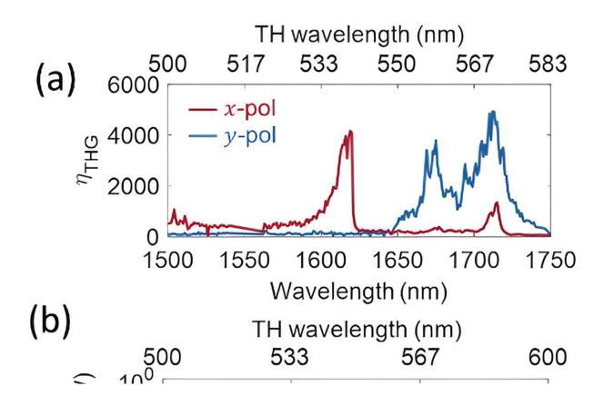
Experimentally measured third-order nonlinear enhancement factor and the corresponding numerical calculation results. Credit: *Opto-Electronic Advances* (2024). DOI: 10.29026/oea.2024.230186
