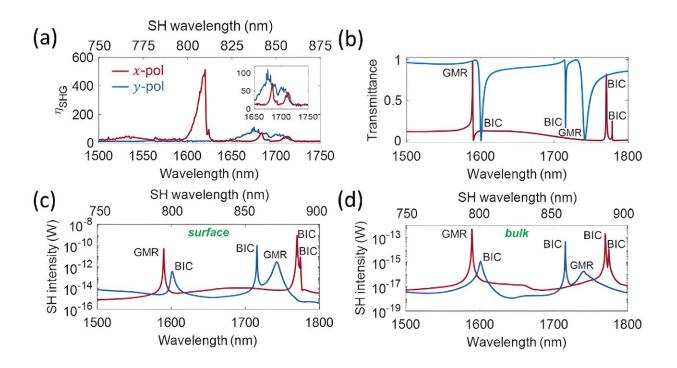
Experimentally measured second-order nonlinear enhancement factor and the corresponding numerical calculation results. Credit: *Opto-Electronic Advances* (2024). DOI: 10.29026/oea.2024.230186
