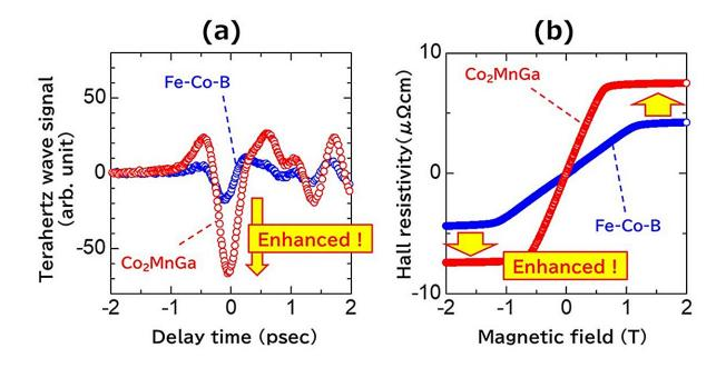
(a) Photo-induced terahertz waves generated from the Weyl magnet: cobalt–manganese–gallium Heusler alloy (Co<sub>2</sub>MnGa) thin film observed in this study. (b) Anomalous Hall effect observed in the corresponding thin film sample. Credit: Shigemi Mizukami
