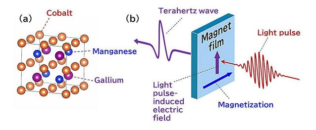
(a) Weyl magnet: schematic diagram of a crystal of cobalt–manganese–gallium Heusler alloy (Co<sub>2</sub>MnGa). (b) Light-induced terahertz waves. Credit: Shigemi Mizukami
