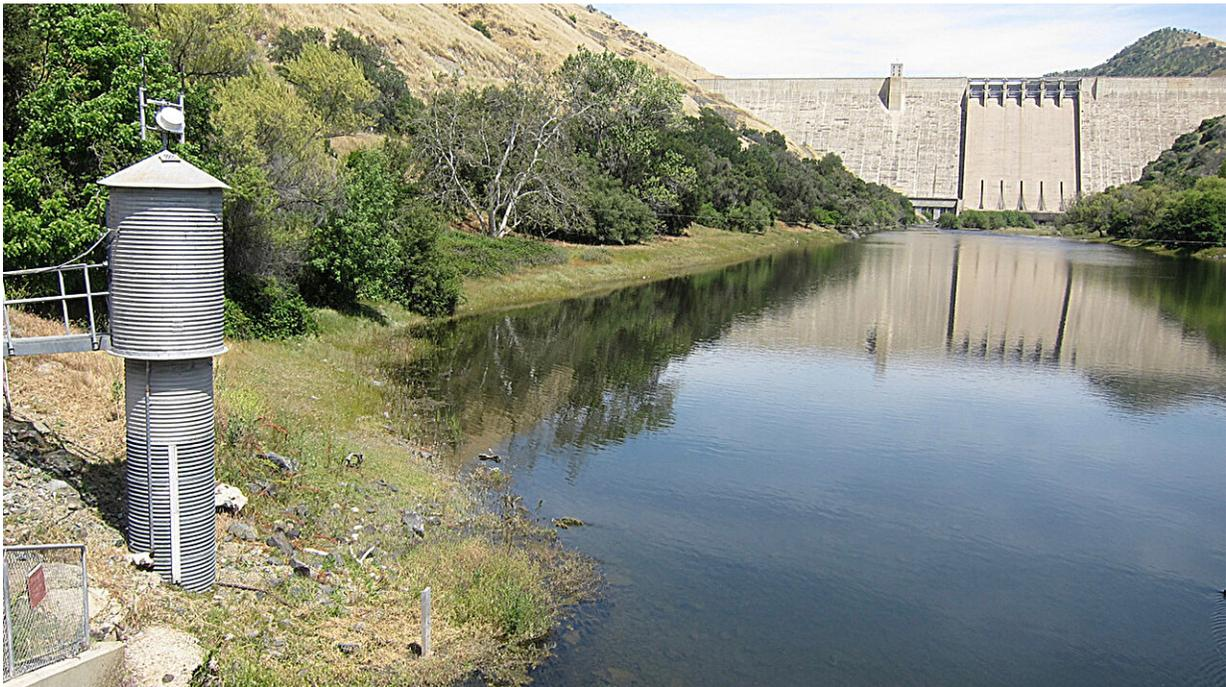
A United States Geological Survey stream gauge measures and records the level of California's Kings River near the Pine Flat Dam in the Central Valley. Credit: University of California - Berkeley
