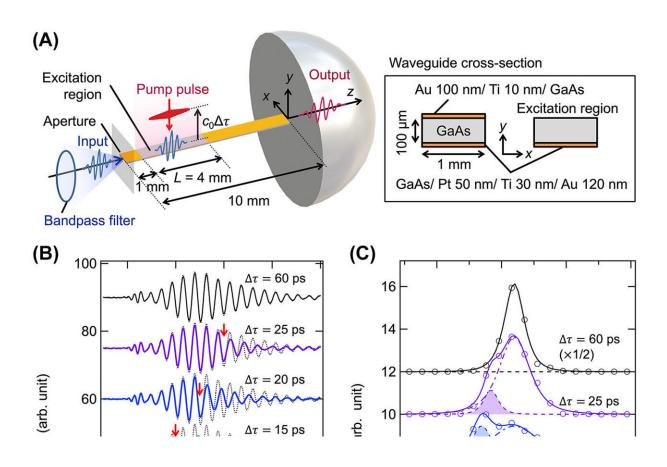
Experimental setup and observed terahertz waves. Credit: *Nanophotonics* (2024). DOI: 10.1515/nanoph-2024-0010
