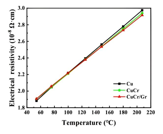
The resistivity versus temperature curves of pure Cu, CuCr alloys and CuCr/Gr wires were tested to determine the effect of Cr and graphene incorporation on resistivity. Credit: *CES Transactions on Electrical Machines and Systems* (2024). DOI: 10.30941/CESTEMS.2024.00009
