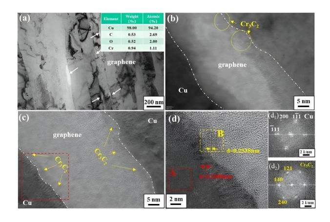
Graphene is distributed along the grain boundaries of the fiber particles, and  $Cr_3C_2$  nanoparticles are pinned at the interface between copper and graphene. Credit: *CES Transactions on Electrical Machines and Systems* (2024). DOI: 10.30941/CESTEMS.2024.00009
