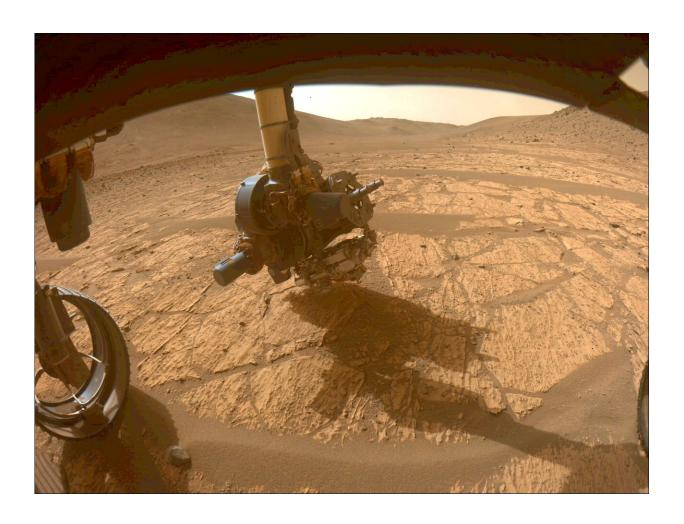
This image of NASA's Perseverance rover gathering data on the "Walhalla Glades" abrasion was taken in the "Bright Angel" region of Jezero Crater by one of the rover's front hazard avoidance cameras on June 14. The WATSON camera on the SHERLOC instrument is closest to the Martian surface. Credit: NASA/JPL-Caltech
