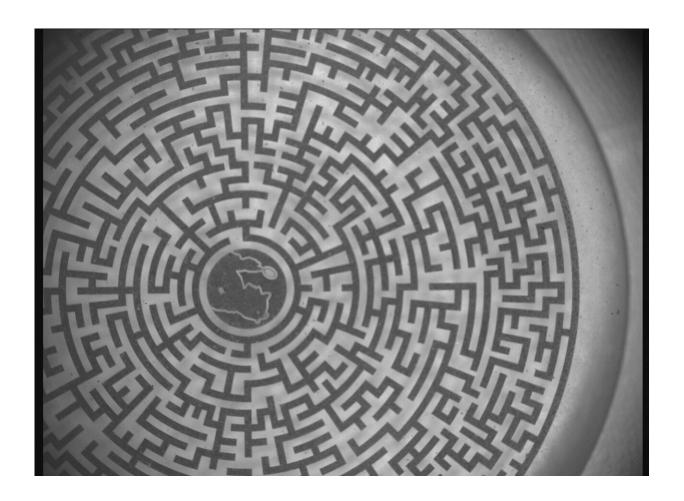
Perseverance's team used the SHERLOC instrument's Autofocus and Context Imager to capture this image of its calibration target on May 11 to confirm an issue with a stuck lens cover had been resolved. A silhouette of the fictional detective Sherlock Holmes is at the center of the target. Credit: NASA/JPL-Caltech
