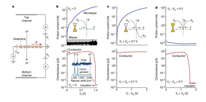
Selective control of proton transport and hydrogenation in double-gated graphene devices. Credit: *Nature* (2024). DOI: 10.1038/s41586-024-07435-8
