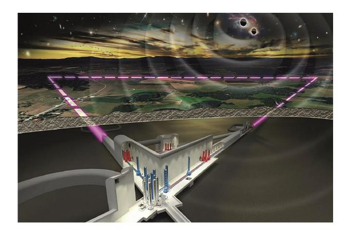
The Einstein Telescope is being built around 250 meters underground. With interferometers in the three tunnels, each ten kilometers long, it will measure collisions of black holes in the early universe. Credit: NIKHEF
