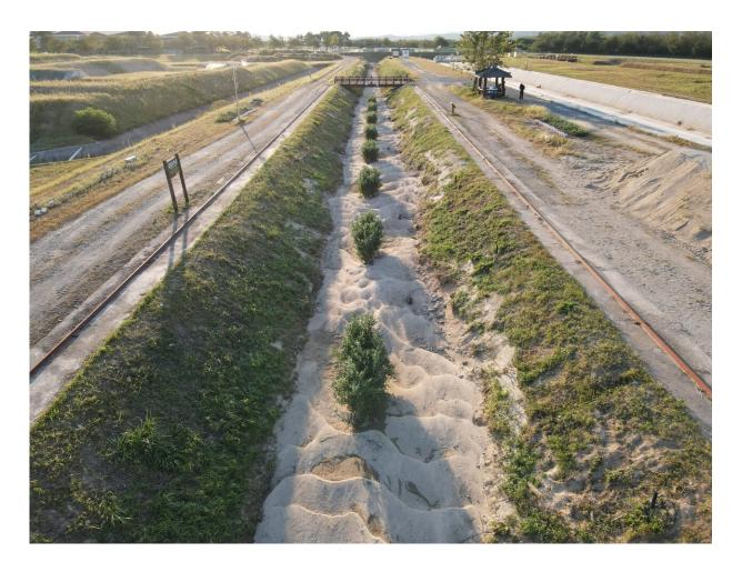
Bedform changes after water discharged in the stream-scale experiment channel with multi patches of vegetation. Credit: Korea Institute of Civil Engineering and Building Technology(KICT)
