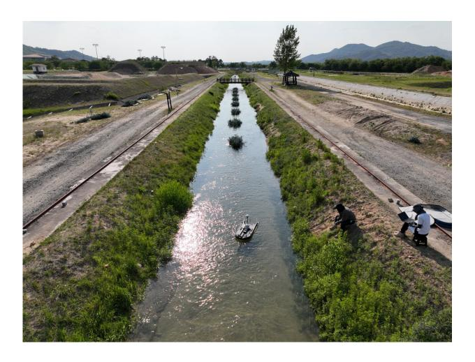
Experimental set-up and discharge measurement during water flows for estimating flow resistance coefficient of woody riparian vegetation patches. Credit: Korea Institute of Civil Engineering and Building Technology(KICT)
