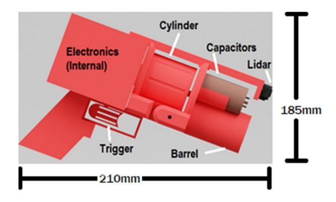
Labeled diagram of the dart launcher, with the placement of primary components. Credit: *Technologies* (2024). DOI: 10.3390/technologies12050069
