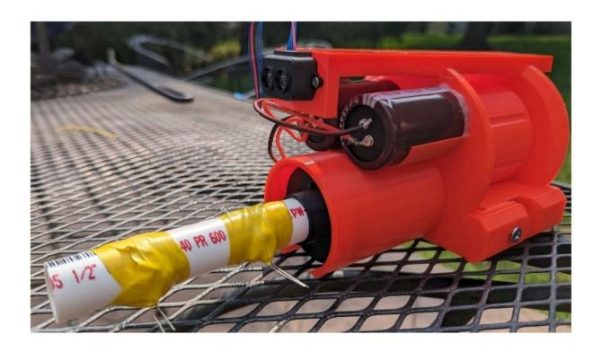
Partial launcher assembly and integrated chronograph in live testing configuration. Credit: *Technologies* (2024). DOI: 10.3390/technologies12050069
