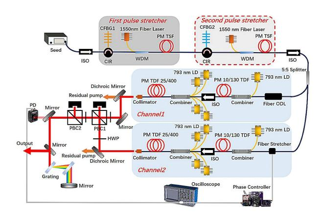
Experimental Setup of the CBC system based on two channels of all-PM TDF-CPA. Credit: *Frontiers of Optoelectronics* (2024). DOI: 10.1007/s12200-024-00117-3
