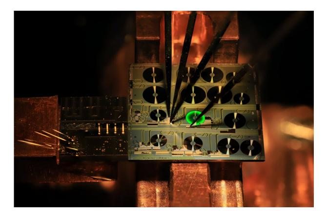
Optical image of a hybrid integrated erbium-doped photonic integrated circuitbased laser, providing fiber-laser coherence and previously unachievable frequency tunability. Credit: Yang Liu (EPFL)
