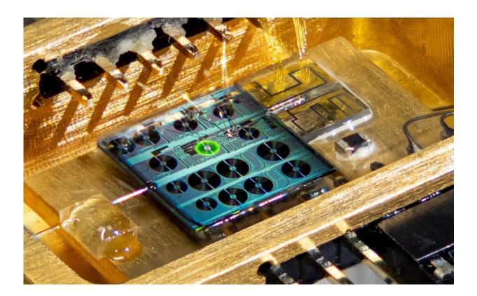
Optical image of a fully-packaged hybrid integrated erbium-laser based on silicon nitride photonic integrated circuit, providing fiber-laser coherence and previously unachievable frequency tunability. Credit: Andrea Bancora and Yang Liu (EPFL)
