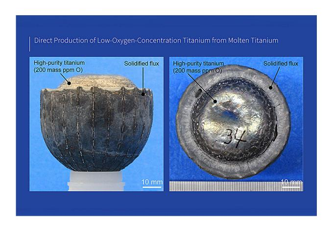
Researchers from the Institute of Industrial Science, The University of Tokyo, have efficiently removed oxygen from high-oxygen-concentration titanium, which might help reduce the production cost of an otherwise versatile metal. Credit: Institute of Industrial Science, The University of Tokyo
