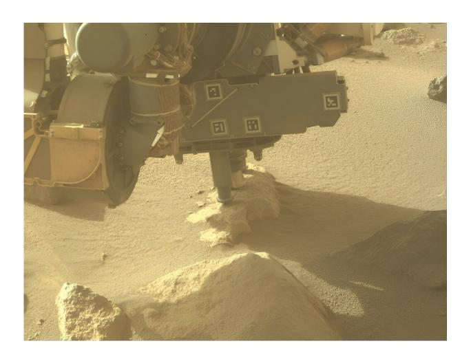
Abrading Old Faithful Geyser: On Sol 1151 (May 16, 2024), Perseverance abraded a carbonate-bearing rock called Old Faithful Geyser in the Western Margin Unit. This activity was captures by the rover's Left Hazard Avoidance Camera (HAZCAM). Credit: NASA/JPL-Caltech
