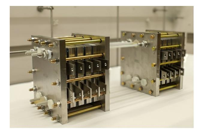
Feng Jiao's two-step system for carbon dioxide (CO2) electrolysis works by converting CO2 into carbon monoxide (CO), then processing CO into multicarbon products like ethylene and acetate, which can be used in the plastics and food industries. Credit: Feng Jiao
