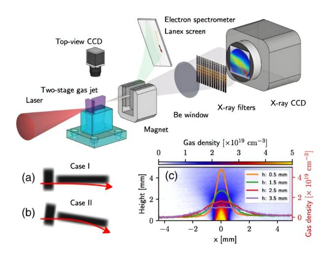
Experimental setup. A laser pulse was focused on a two-stage gas jet to produce electron and betatron x rays. (a) and (b) The schematic of the laser-target geometry in the two cases, respectively. The red arrows represent the laser trajectories. (c) Measured averaged transverse neutral gas density distribution at a backing pressure of 4.1 MPa and gas density profiles at different heights above the nozzle for the accelerator. Credit: *Physical Review Letters* (2024). DOI:
