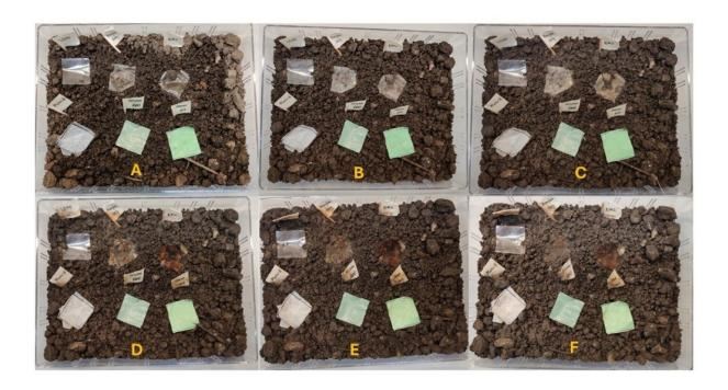
Experiments on the degradation of different plastic materials. Top left is a common LDPE plastic film. Top center and right are the researchers' amylose-based bioplastic and a plastic made from corn starch, respectively. At the bottom are three different bags made from conventional bioplastics. A) shows the start of the experiment. B) shows the degradation after 8 days, C) the degradation after 11 days, D) 21 days E 41 days and F) shows the degradation after 54 days. Credit: Andreas Blennow
