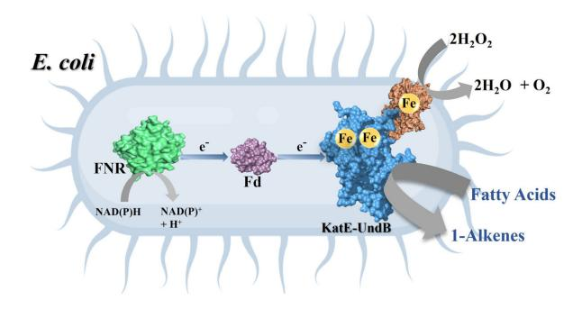
Engineered whole cell biocatalyst for efficient 1-alkene production. Credit: Tabish Iqbal
