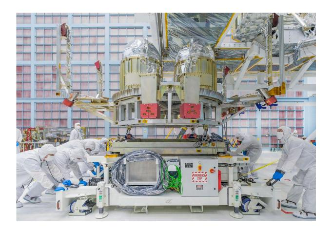
In this photograph from Feb. 29, 2024, at NASA's Goddard Space Flight Center in Greenbelt, Md., the Roman Space Telescope's propulsion system is positioned by engineers and technicians under the spacecraft bus. Engineers used augmented reality tools to prepare for the assembly. Credit: NASA/Chris Gunn
