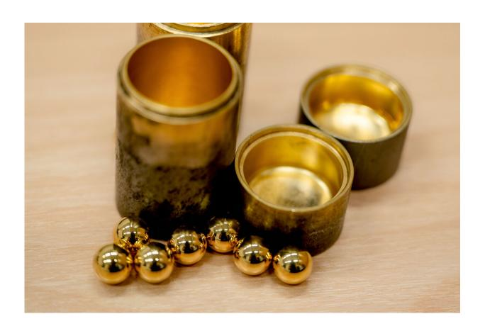
Gold-lined grinding bowls can catalyse reactions without solvents. Credit: RUB, Marquard
