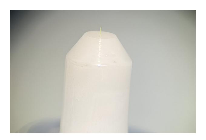
Image of fiber connector tip, with diminutive photonic lantern printed directly onto the fiber facet. Credit: Yoav Dana
