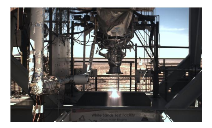
Orion Main Engine injector test engine firing. Credit: NASA
