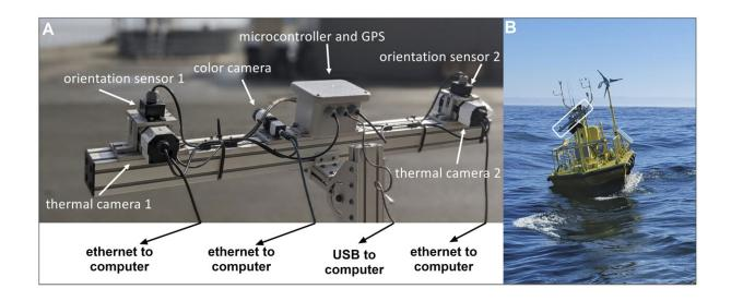
Close-up of ThermalTracker-3D offshore prototype system sensors (A) and a depiction of this system during deployment in 2021 on a WindSentinel buoy (outlined in a white bounding box) (B). Credit: *Frontiers in Marine Science* (2024). DOI: 10.3389/fmars.2024.1346758
