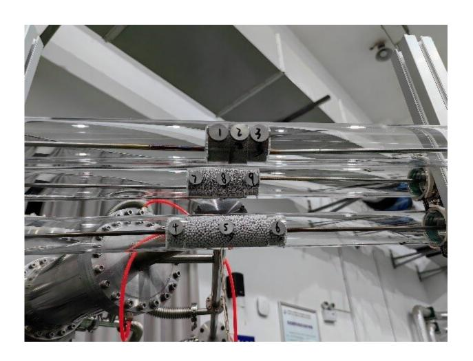
Sample layout for 14 MeV fusion neutron irradiation. Credit: FU Xuewei
