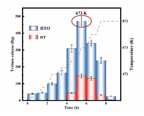
Tritium release curve of Li<sub>2</sub>TiO<sub>3</sub> in various temperature. Credit: FU Xuewei
