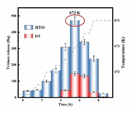
Tritium release curve of Li<sub>2</sub>TiO<sub>3</sub> in various temperature. Credit: FU Xuewei
