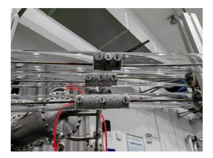
Sample layout for 14 MeV fusion neutron irradiation. Credit: FU Xuewei
