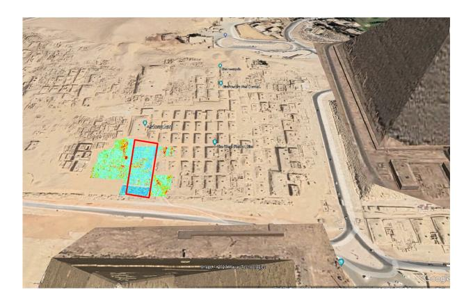
Location of the survey area projected on Google Maps. The red rectangle shows the area of the initial survey. The color figure shows the horizontal profile of GPR. View is to the north. Credit: *Archaeological Prospection* (2024). DOI: 10.1002/arp.1940
