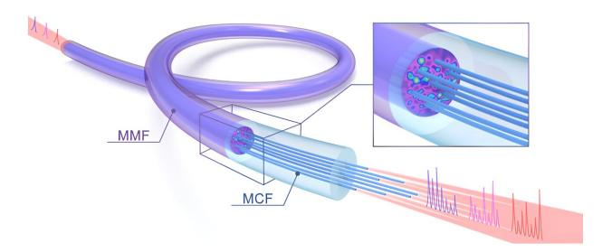
the input pulse is mapped into a speckle pattern through the MMF. Then, the MCF samples the output pattern into a pulse sequence. The seven cores of the MCF are extended in different lengths to avoid overlapping. Credit: Zheng Gao, Ting Jiang, Mingming Zhang, Yuxuan Xiong, Hao Wu, and Ming Tang.
